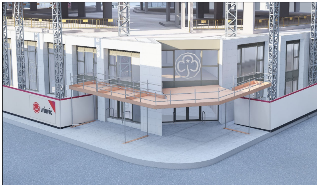
Scaffold protection over the Main Entrance and Main Hall Fire Escape (Indicative only, the true layout/supports are subject to final design requirements)
